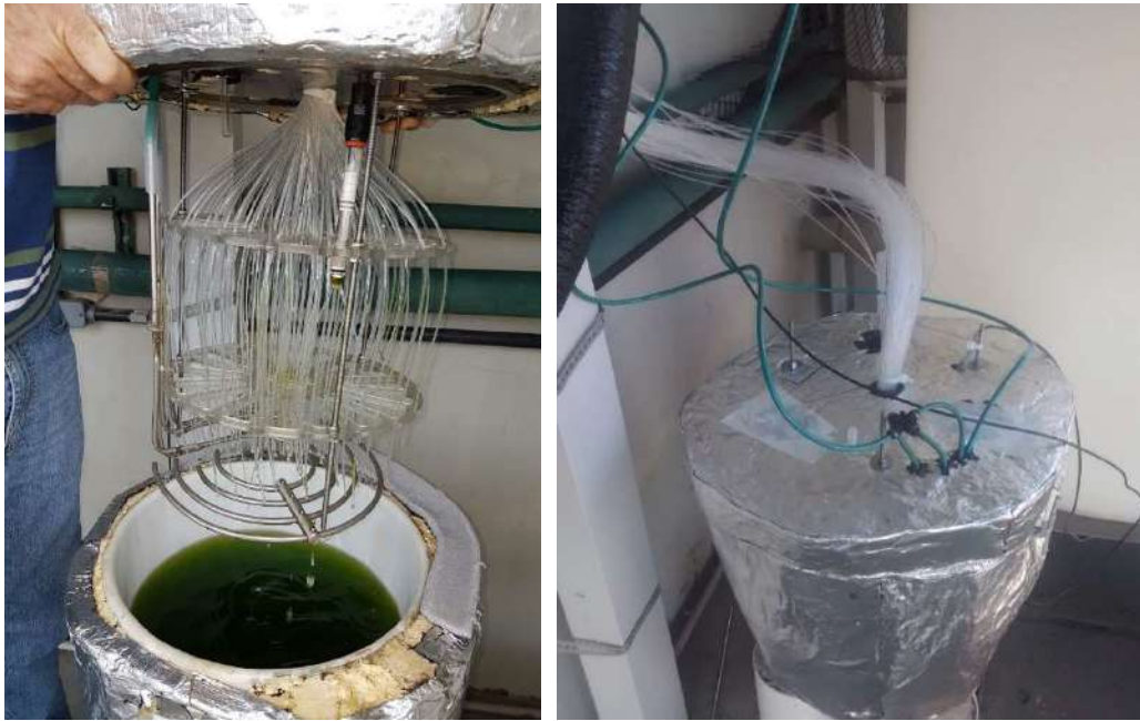
Figure 9. Left: Fiber arrangement inside de 30-liters PBR. The lower serpentine contains holes for aeration and CO 2 supply. The cylinder at top is the light sensor. Right: PBR closed, at the beginning of the cultivation. In both pictures it is possible to notice the thermal protection around the PBR to protect the cell culture against outside thermal oscillations.
