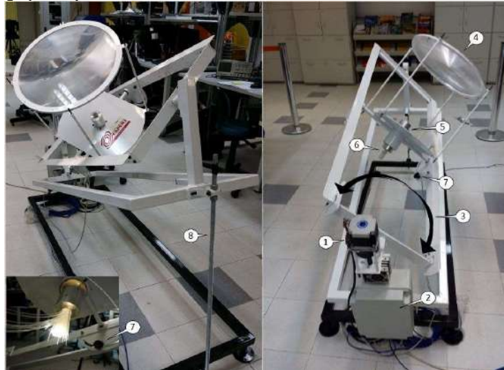
Figure 5. Right: The solar tracker being assembled in laboratory. 1) Stepper motor, driven by the control box (2). 3) Rotatory frame the follows the Sun. 4) Fresnel lens. 5) Support of POF bundle at focus point of the lens. 6). POF bundle. 7) Declination adjustment. Left: Another view showing the inclination adjustment of the local latitude (8). Lower Left: POF bundle support in test with short fibers illuminated by an artificial light.
