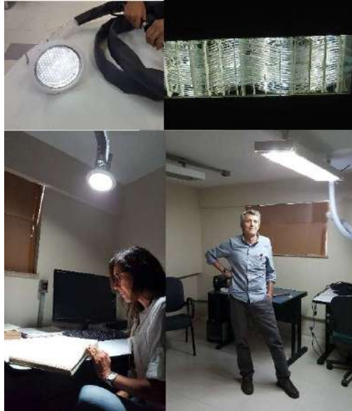
Figure 15. Luminaires developed and their illumination effect. Top left: Spot luminaire; Bottom left: Illumination obtained with the spot luminaire; Top right: Diffuse luminaire; Bottom right: Illumination obtained with diffuse luminaire.
