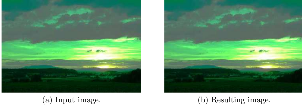
Figure 3.27: (a) Digital FPTMO output image, after demosaicing, which is an input for the White Patch white-balance algorithm; (b) White Patch algorithm result.
