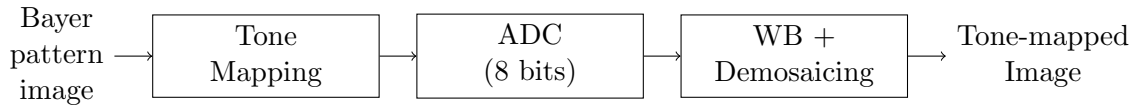
Figure 3.39: Cascade of image processing stages that support focal-plane tone mapping. The FPTMO itself is denoted by the “Tone Mapping” block.
