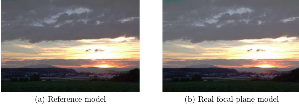
Figure 3.33: Images resulting from (a) the reference model and (b) the real focal-plane model. Each model uses a different white-balance approach.
