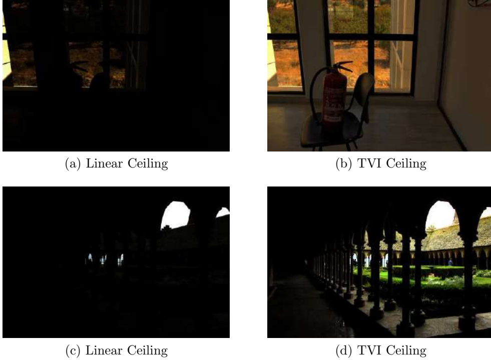
Figure 2.25: Images resulting from the Ward histogram adjustment tone-mapping operator, using different procedures to avoid exaggerated contrast in the tone-mapped images.
