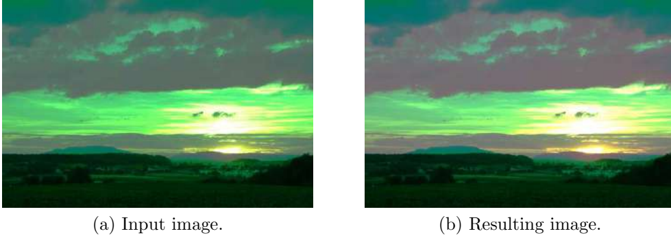
Figure 3.29: Application of the RAWB white-balance algorithm to the tone-mapped image after demosaicing.
