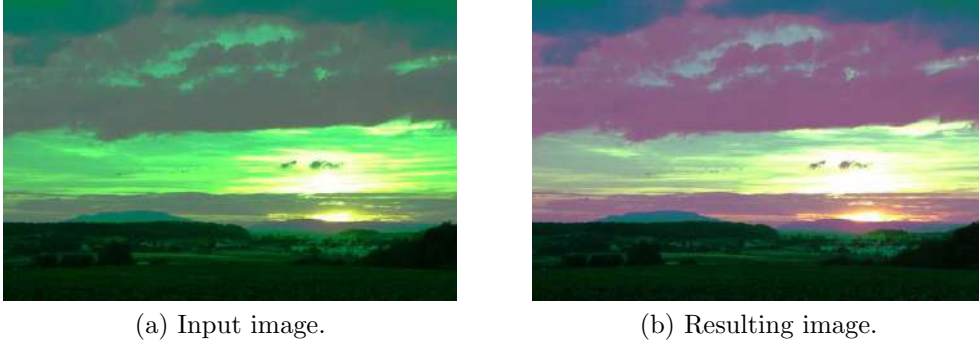
Figure 3.25: Application of the Gray World white-balance algorithm to the tone-mapped input image, after the demosaicing.
