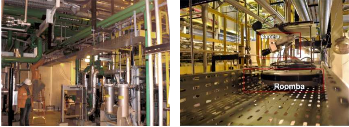
Figure 3.2: Pictures taken at the facility where the VDAO sequences were recorded. The left picture shows an overview of the industrial environment and the hanging rail. The right one exhibits a close shot of the iRobot TM Roomba on the rail track with the mounted camera.
