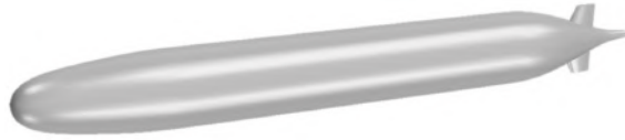
Figure 2.2: The UV under consideration equipped with a vertical rudder in the stern region
