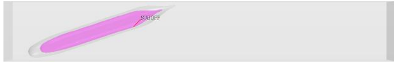
(b) The regions around the UV where the mesh is refined in drift tests for \beta = 18.11^\circ
