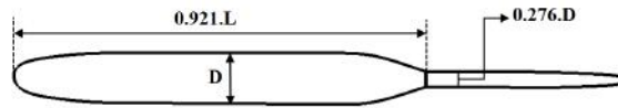
Figure 2.16: The axisymmetric SUBOFF bare hull model with the support used by ETEBARI et al. [41]
