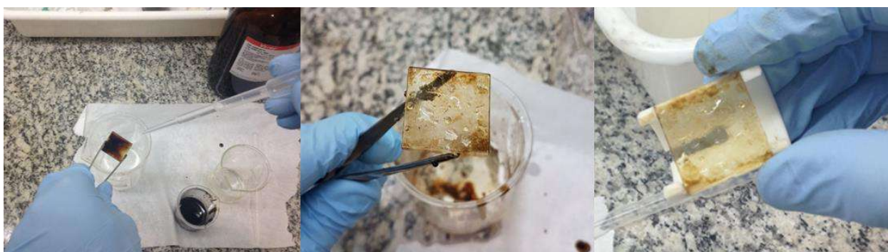
Figure 4.2. Excess bulk oil cleaning by applying solvent (cyclohexane).
