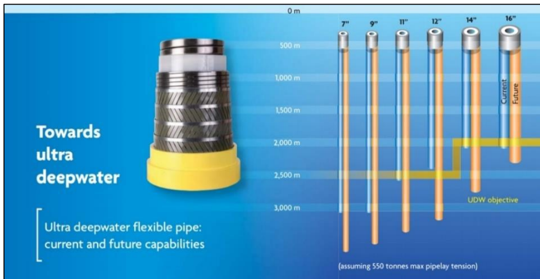
Figure 6 – Flexible pipe with CFA wires, current and future water depth capacity by internal diameter (from DO et al. [5]).
