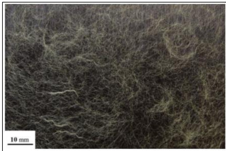
Figure 22 – Microscopy of aramid short fiber tissue [32].
