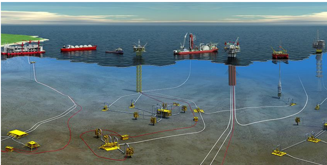
Figure 3 – Subsea architecture of flexible and rigid risers [8].
