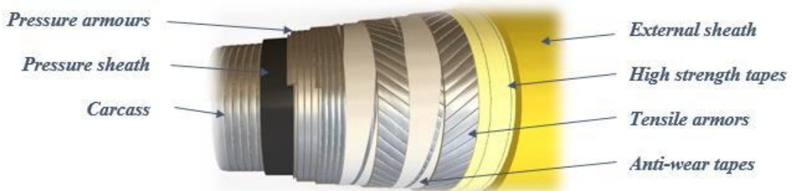
Figure 5 – Typical layers of flexible riser.
