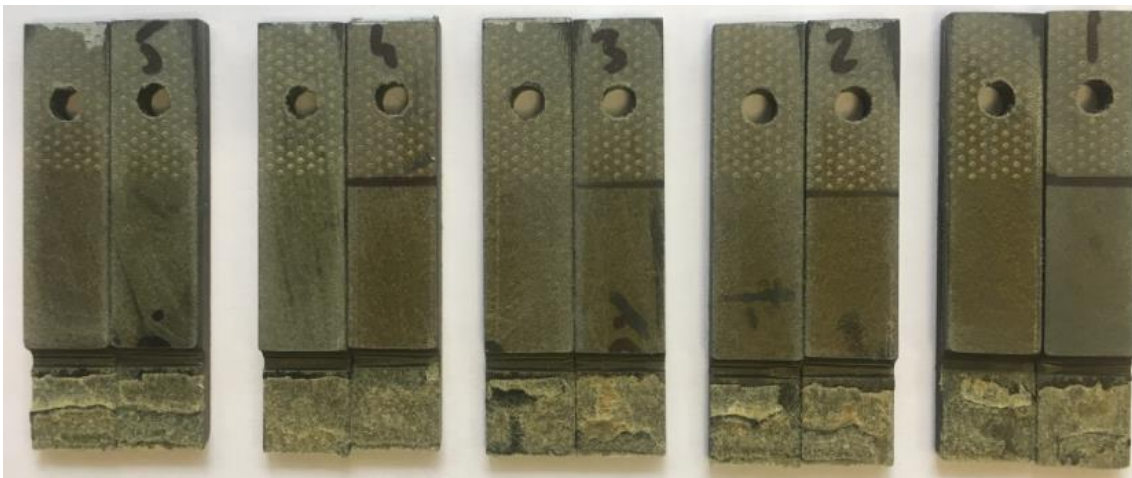
Figure 93 – Lap shear samples after testing showing fracture surfaces at the bottom of picture. Rupture in substrate, at the first ply of the CFA, that is at Mat level.
