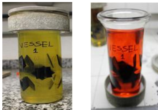
Figure 19 – Immersion vessel of NBR in Diesel (a) before immersion (B) after 1 week of immersion
