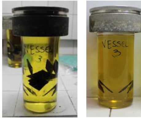
Figure 23 - Immersion vessel of HNBR (a) before and (b) after 1 week of immersion in Diesel
