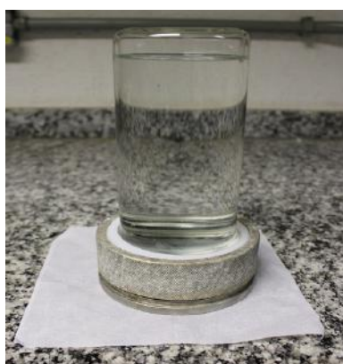
Figure 12 – Immersion vessel assembled during leakage test
