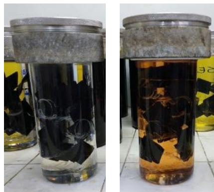
Figure 20 – Immersion vessel of NBR in Xylene (a) before and (b) after 1 week of immersion
