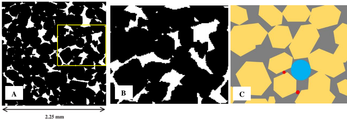
Figure 7: a) Thin-section Fontainebleau sandstone. The pore space is shown in white and the grain in black. Reproduced from Okabe and Blunt, 2005. b) Cropped area from yellow square in picture a. c) Drawing of the representation of the pore space with simplified geometries. The grains are represented in yellow and pore space in gray. Blue sphere represents a pore and in red the throats.
