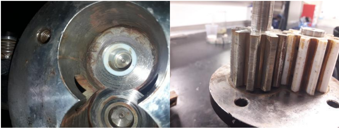
Figure 4.42: Erosion and misalignment presented in the first pump
