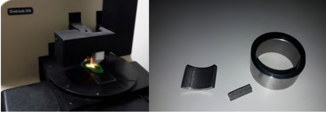
Figure 3.2: Profilometer and sections to roughness measurements
