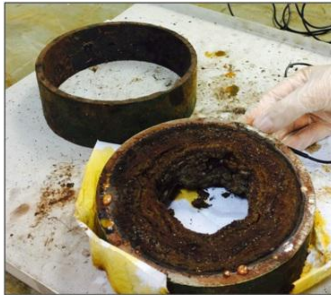
Figure 1.1: Scale formation in actual pipe cross-section, Source: Subsea Technology Laboratory, COPPE / UFRJ.
