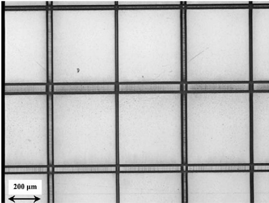
Fig. 2.8 – Overview of a partially-regular micromodel with pore dimensions equal in shape and varying in size [75].
