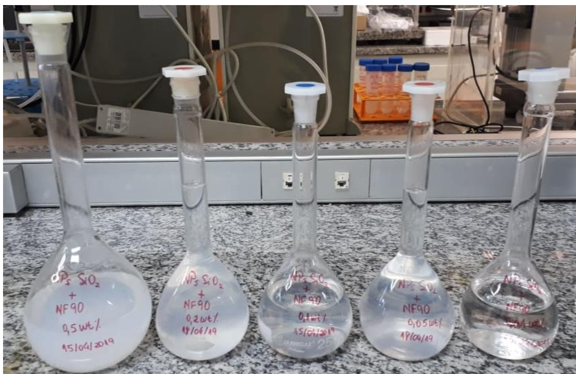
Fig. 3.4 – Prepared SiO 2 nanofluids in varied concentrations. From left to right: 0.5 wt.%, 0.2 wt.%, 0.1 wt.%, 0.05 wt.%, 0.01 wt.%.
