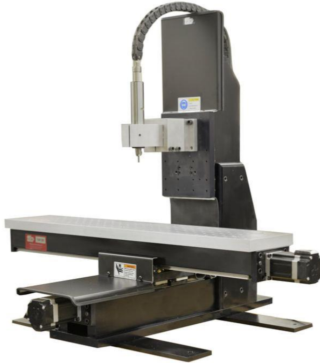
Fig. 3.2 – Microdrill CNC milling machine used to fabricate the micromodel molds. A tungsten carbide micro tool cut through an acrylic substrate by the means of a program code. The removed material from the acrylic mold represent the grains of the pore-network [142].
