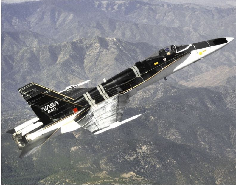
Figure 1.4: The F-18 aircraft was widely studied at NASA for achieving an angle of attack as high as 70 degrees 1 .
