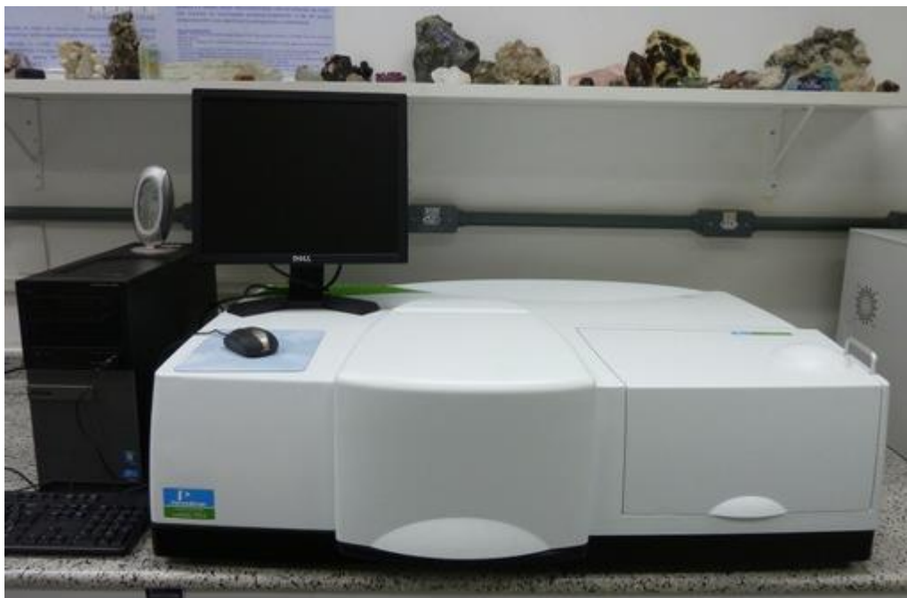
Figura 24 – Espectrômetro UV – VIS – NIR Perkin Elmer Lambda 750S
