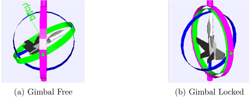
Figure 25: Illustration of the gimbal lock limitation of Euler Angles representation of attitude.
