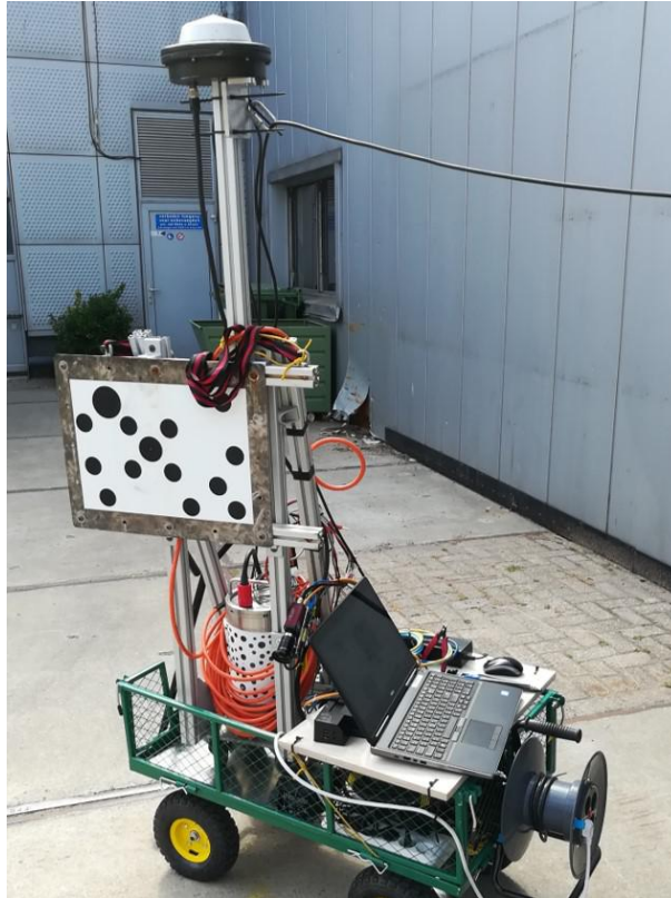
Figure 20: Equipment used for the third dataset. On top, the antenna. At bottom-left, the Rovins. Between the computer and the Rovins, the Camera mounted to the DMU-11. Under the computer, the StarPort and StarPack.
