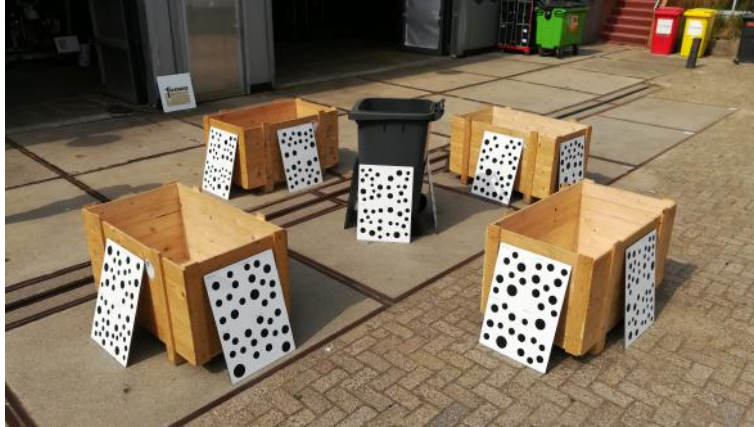
Figure 22: Arrangement of patterns for third dataset, allowing a circular path of about 8 meters of diameter.
