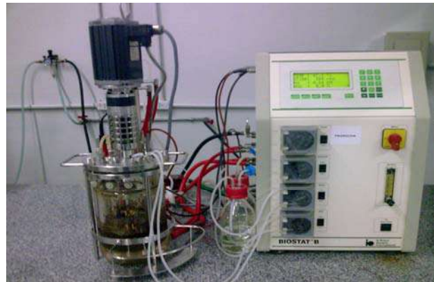
Figura IV.15: Biorreator BIOSTAT B (B. Braun International) durante o processo SSF
