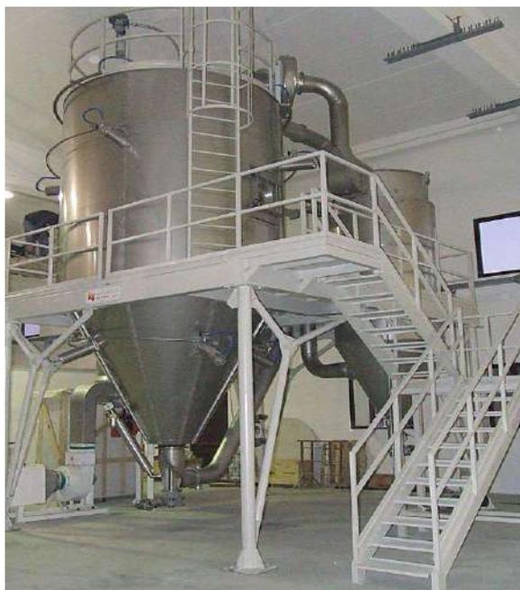
FIGURA 15 – EXEMPLO DE UM “SPRAY DRYER” (FONTE: CHANGZHOU HENGCHENG FIRST DRYING EQUIPMENT CO., LTD.).
