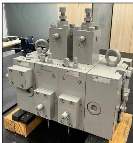
Figura 12 - Main Control Valve
