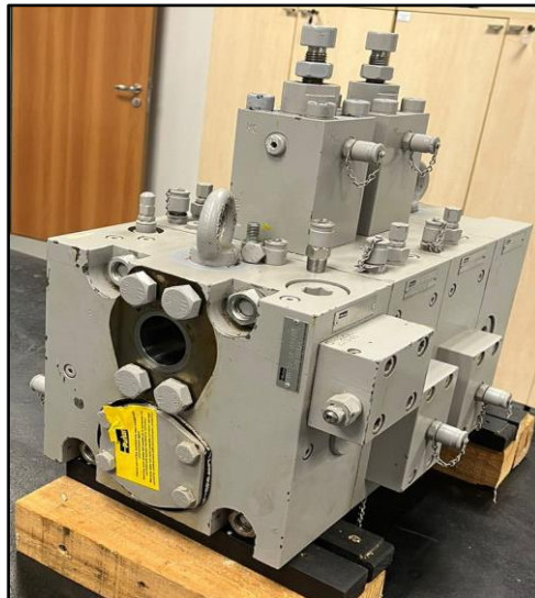
Figura 14 - Main Control Valve
