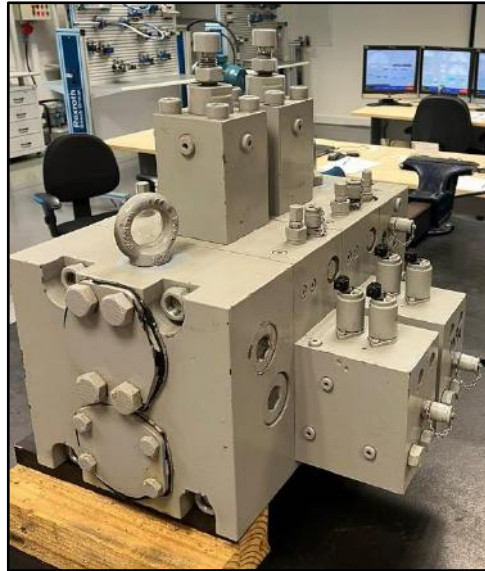
Figura 13 - Main Control Valve
