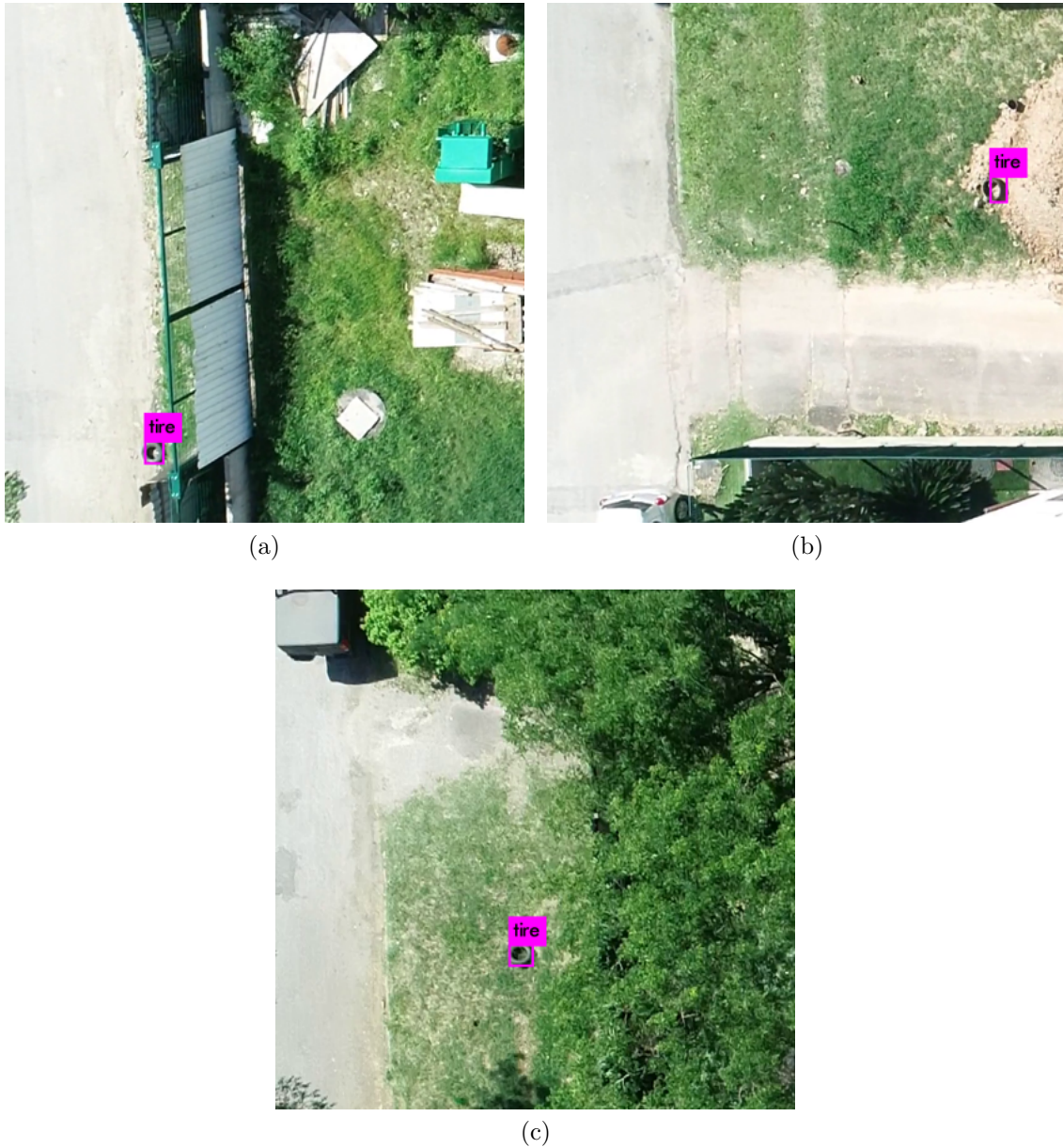
Figure 5.6: Examples of YOLO (blur and blend) detections on video BLI3. The tires of Subfigures (b) and (c) are detected by the six networks.
