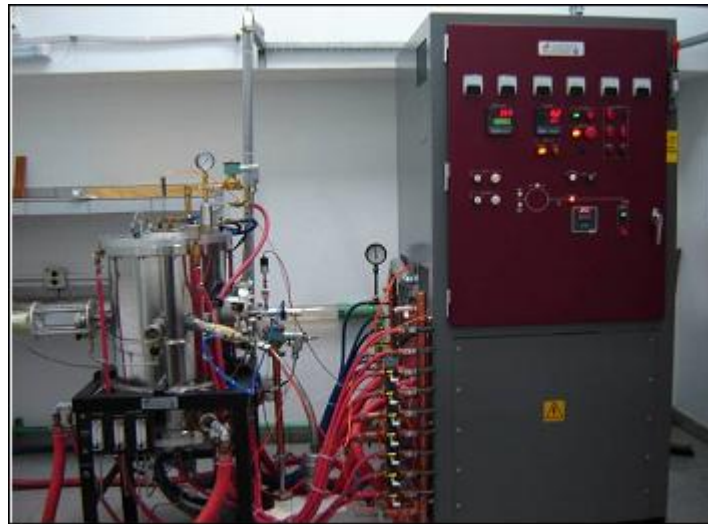
Figura 3 - Forno Series 45 Top Loaded Vacuum Furnaces (Centorr Vacuum Industries)
