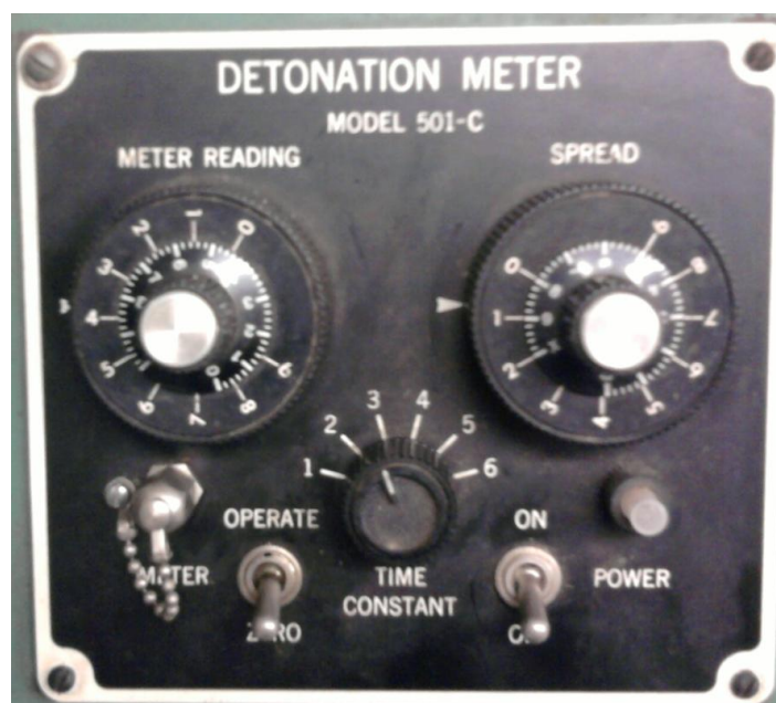
Figura 4.7 - Detonation Meter – Motor CFR-F2
