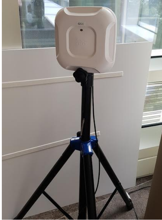
Figure 5 - An example of a WiFi access point placed on top of a tripod stand, to guarantee
