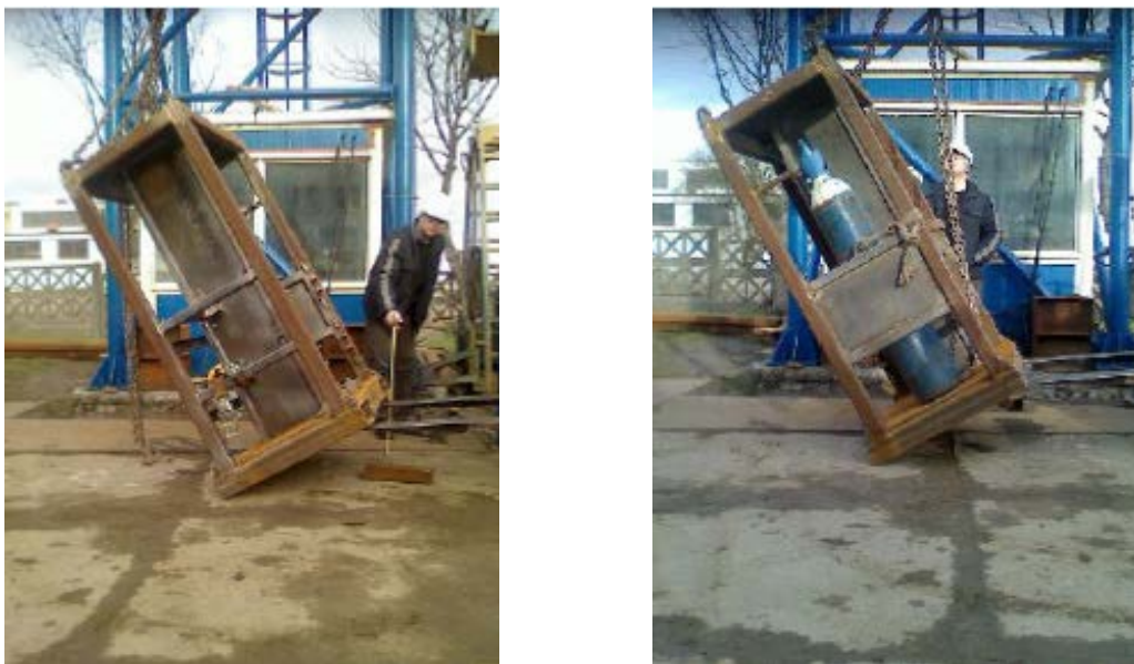
Figura 6.5.1 - Container Offshore no Tilt Test
