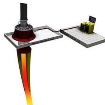
Scheme of a monitoring system for curvature
