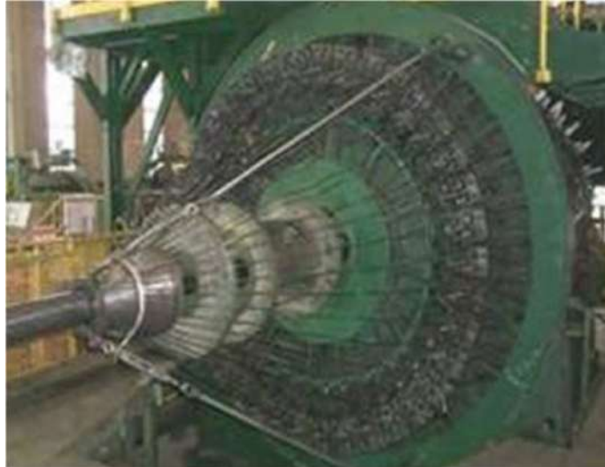
Figure 2.6. Manufacturing process of tensile armors (FACHINI, 2014)
