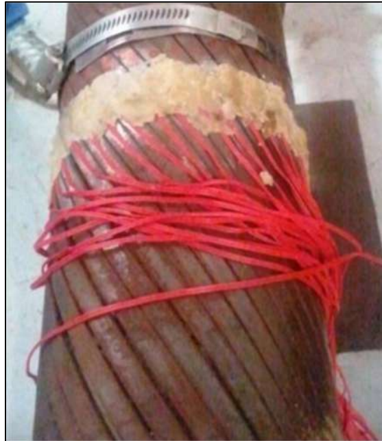
Figure 4.2. Strain gauges installed // outer tensile armors (SOUSA, et al. , 2015)
