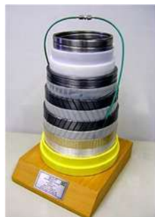
Flexible Pipe ready for Flooding Detection System
