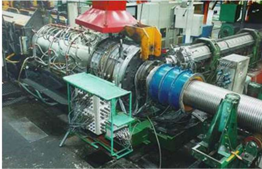
Figure 2.3. Manufacturing process of pressure sheath (FACHINI, 2014)
