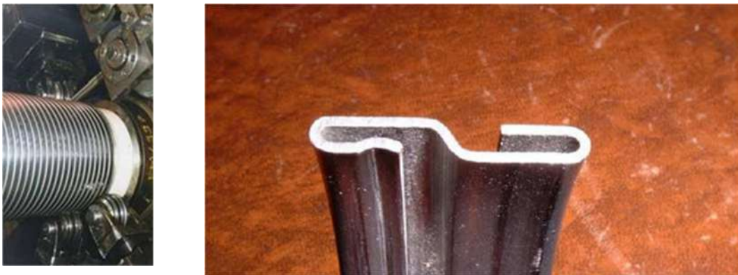
Figure 2.2. Manufacturing process of Carcass (adapted from (FACHINI, 2014))
