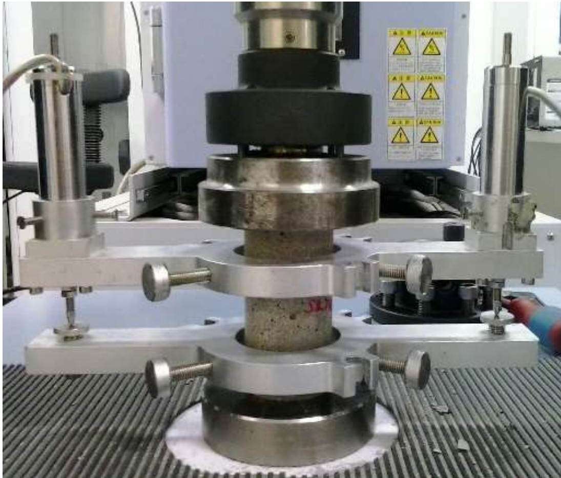
Figure 5-1 Compression test on cylinder specimen with deformation measured by LVDT.
