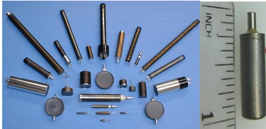
Figura 64 – Diferentes tubos Geiger – Fonte: www.Indinc.com/products/category/34/
