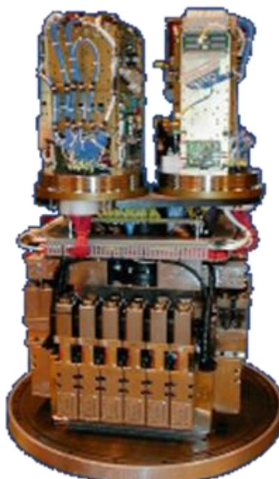
*Figura 46 – Subsea Control Module*
