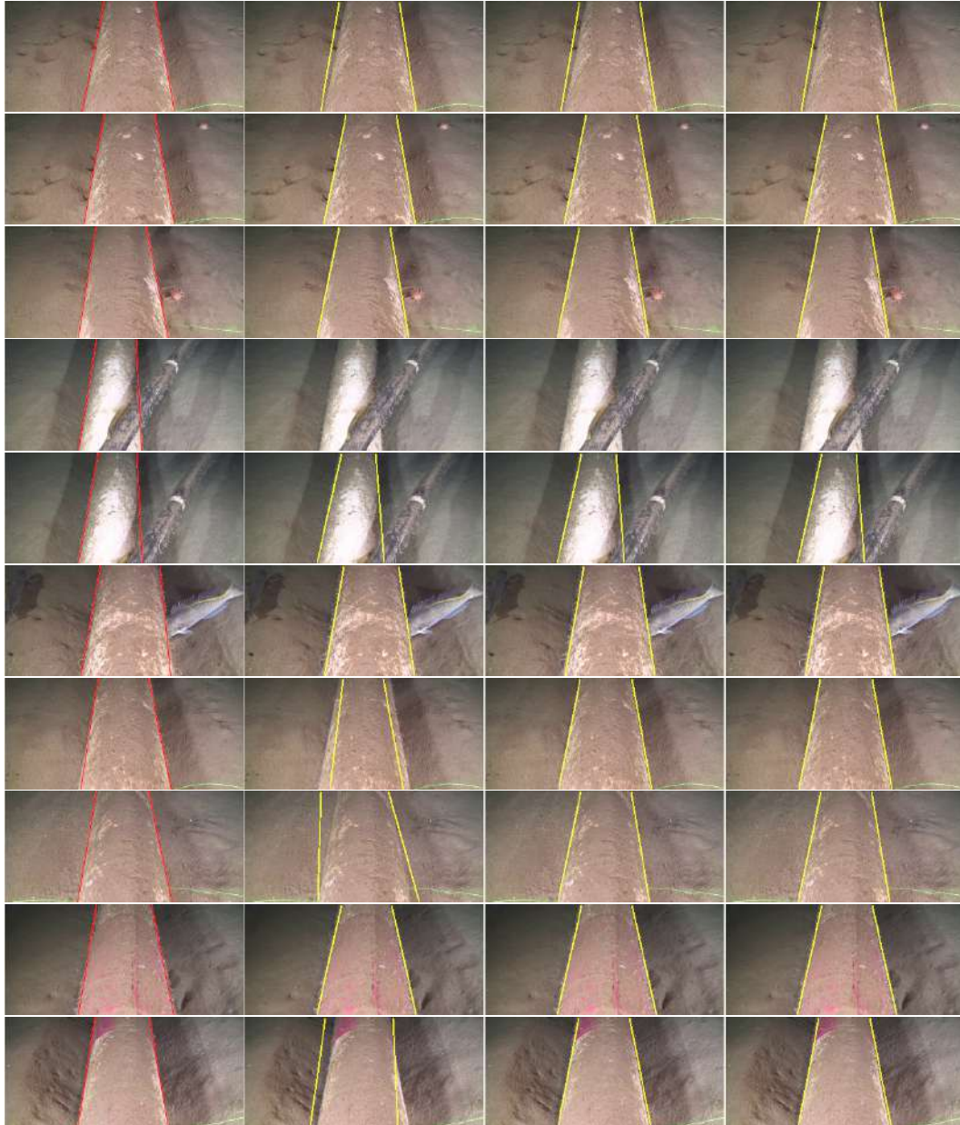
Figure 3.8: Detection example from video 6. From left to right: ground truth (red), tracking using 2, 5 and 9 frames (yellow).
