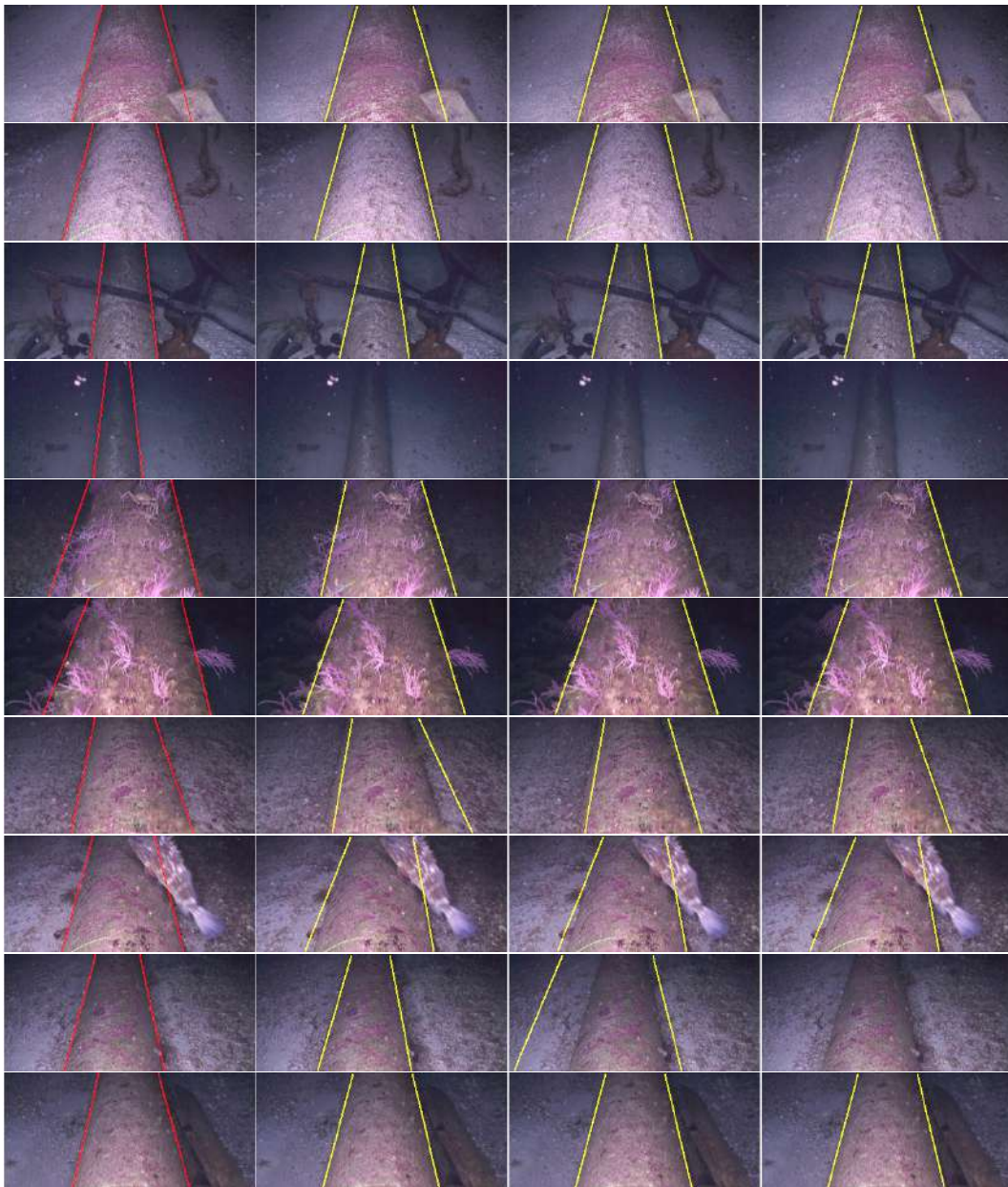
Figure 3.3: Detection example from video 1. From left to right: ground truth (red), tracking using 2, 5 and 9 frames (yellow).
