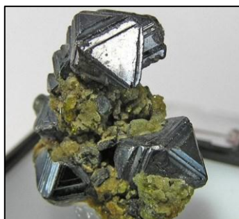
Figura 1: Minério de magnetita ( \text{Fe}_3\text{O}_4 ) na natureza. Fonte: Rob Lavinsky, iRocks.com – CC-BY-SA-3.0, CC BY-SA 3.0, < https://commons.wikimedia.org/w/index.php?curid=10149794 >
