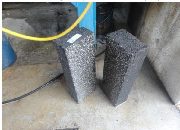
*Figura 33c – Prisma serrado*
