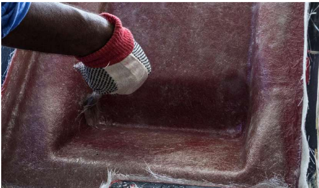
Figura 188. Processo de laminação manual. fonte ( http://signatureproducts.com/our-processes/signature-products-hand-lay-up-process-for-contact-moulding ).
