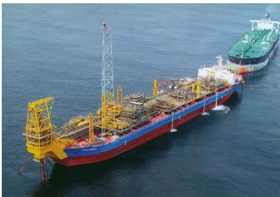
Figura I.1: FPSO ( Floating, Production, Storage and Offloading ) e Navio Aliviador [6]
