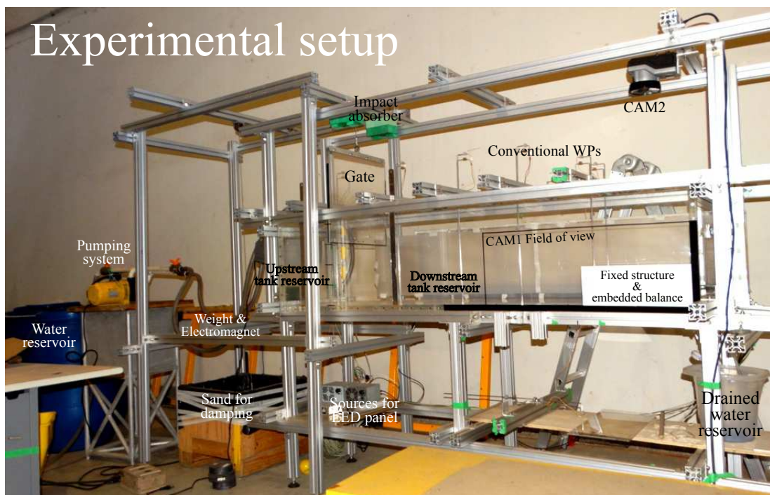
Figure B.1: General view of the complete experimental setup, considering the experiment with the rectangular fixed structure inside the tank.
