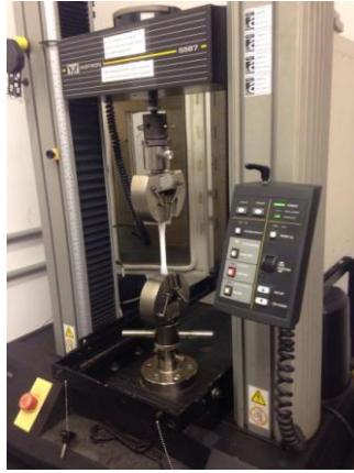
Figure 54. Universal testing machine Instron (model 5567). Laboratory of Materials Processing and Characterization (LPCM) – PEMM / UFRJ.
