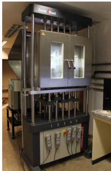
Figure 53. Zwick/Roell machine (Kappa Multistation model) for stress relaxation tests. Laboratory of Materials Processing and Characterization (LPCM) – PEMM / UFRJ.
