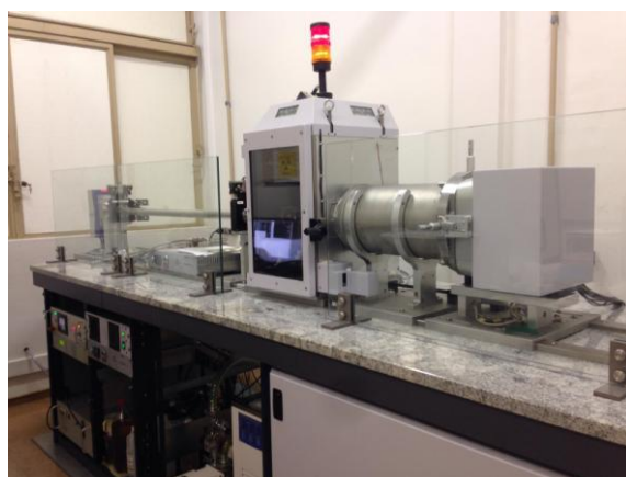
Figure 58. NanoSTAR SAXS system (Bruker AXS) coupled to Cu K\alpha radiation source Xenocs (Genix 3D Cu ULD) and to a Bruker Vantech 2000 detector. Institute of Physics – USP.
