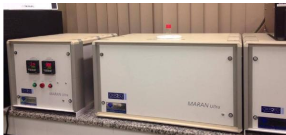
Figure 57. Maran Ultra spectrometer, electromagnetic field of 0.54 T (23.4 MHz for ^1\text{H} ). Institute of Macromolecules Professor Eloisa Mano (IMA) – UFRJ.
