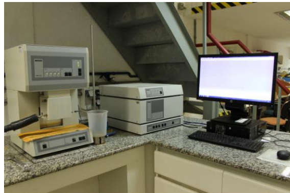
Figure 55. Netzsch DMA 242C instrument. Laboratory of Materials Processing and Characterization (LPCM) – PEMM / UFRJ.
