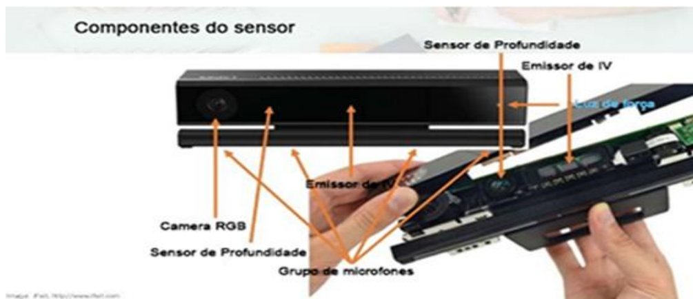
Figura 2.5 – Componentes do sensor Kinect, adaptado de (KERKHOVE, 2014)
