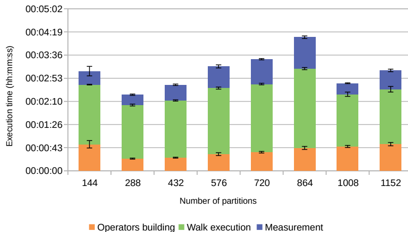
Figure 4.7: Execution times for 10 steps quantum walks on three worker nodes with different number of partitions.
