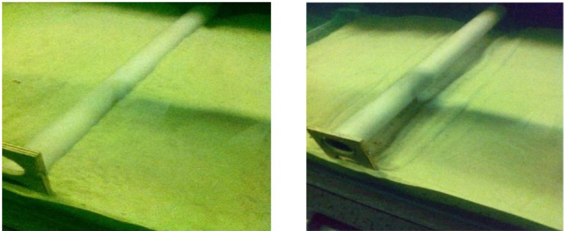
Figure 15 - Reproduction of [16] Experiment with Pipelines: (b) Initial Setup; (c) After 15 minutes of Progressive Waves [17]
