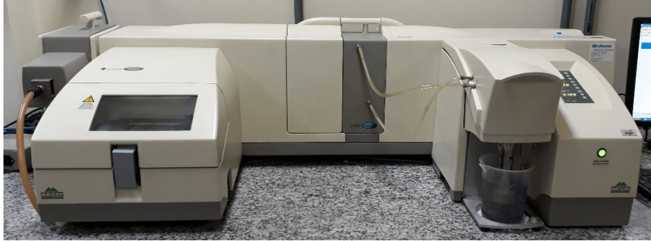
Figura 3.11: Granulômetro a laser Mastersizer 2000 Malvern Instruments
