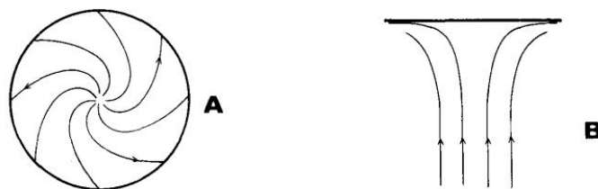
Figure 2.4: Cross section view (A) and side view (B) of the streamlines for the RDE system. Adapted from [8].
