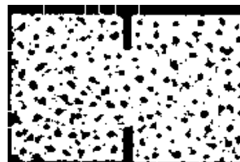
(d) Image after watershed, area filtering, and despeckle.
