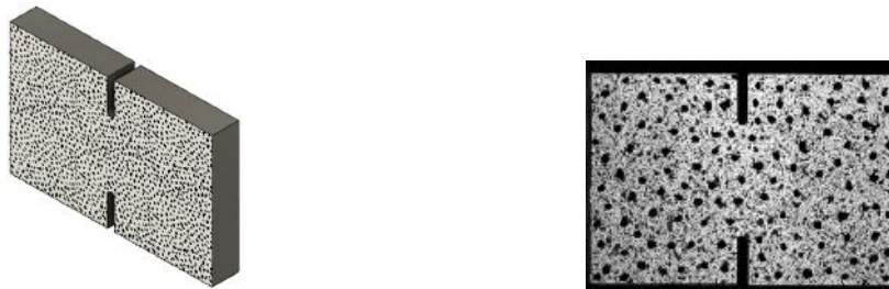
(a) Illustration of a specimen surface. (b) Type II specimen with applied speckle.
