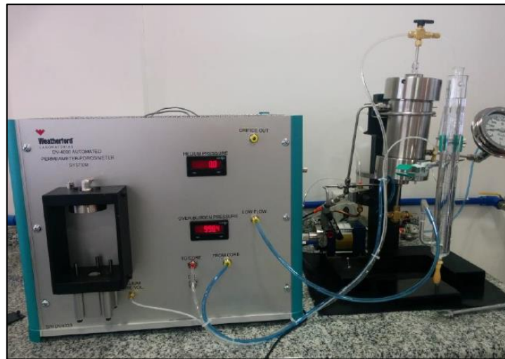
Figure 3-8 – Detail of the DV-4000 porosimeter and permeameter used to obtain the measurements of effective porosity and absolute permeability of the samples studied.
