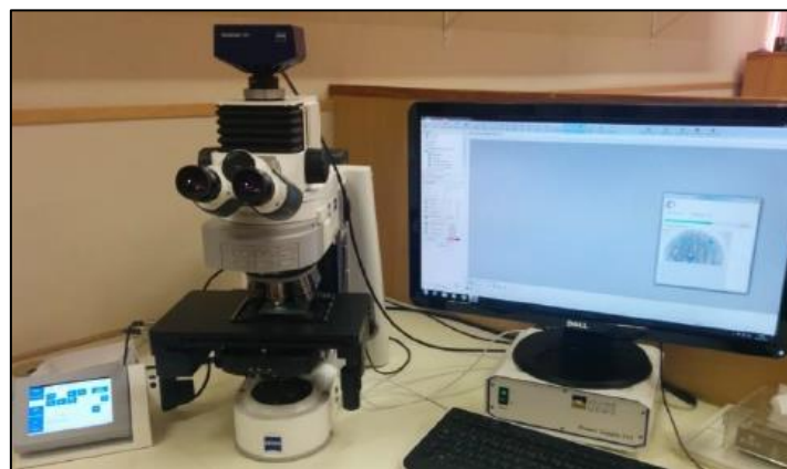
Figure 3-7 – Detail of the Zeiss Imager M2m optical microscope used to evaluate the thin sections of the selected samples.
