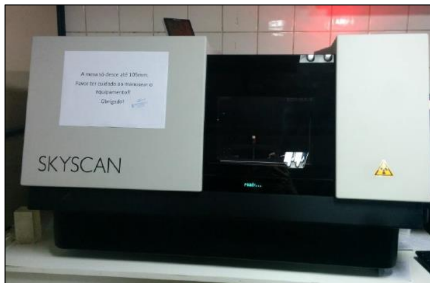
Figure 3-9 – Photograph of X-ray microtomography of Bruker model Skyscan 1173 used to acquire images with different resolutions.
