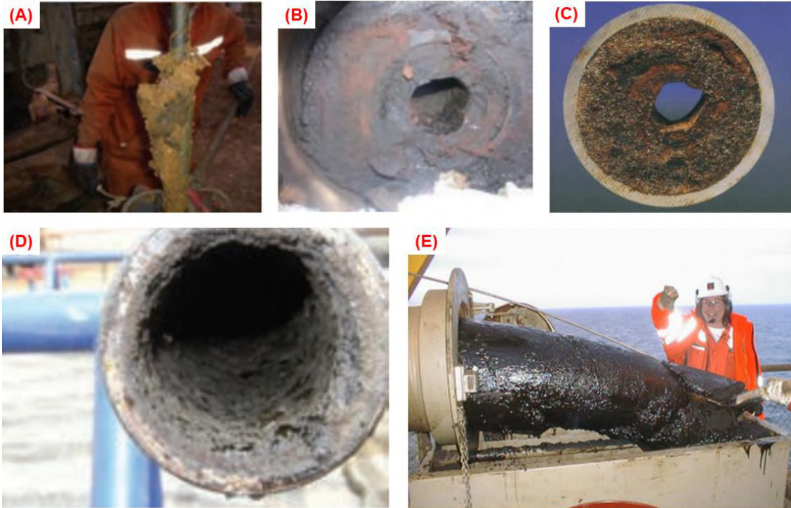
Figure 1 - The consequences of continuous wax deposition on (A) well tubing string, (B, C, and D) cross-section of flow lines, and (E) a pipe from a Norwegian production platform (extracted from Tukenov [9], with permission).
