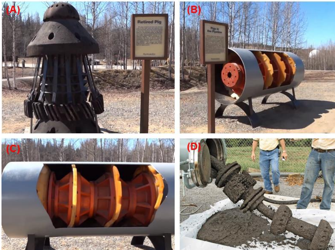
Figure 3 - Pipeline Inspection Gauges or PIGs are launched and retrieved at pump stations and travel through the pipeline with the moving oil. (A) retired PIG equipment of 1,160 kg, (B and C) a lighter and softer polyurethane PIG and (D) the resulting of pigging operation. Images extracted from "Trans Alaska Oil Pipeline Tour" video, available at https://www.youtube.com/watch?v=_OrAmGOFOEk
