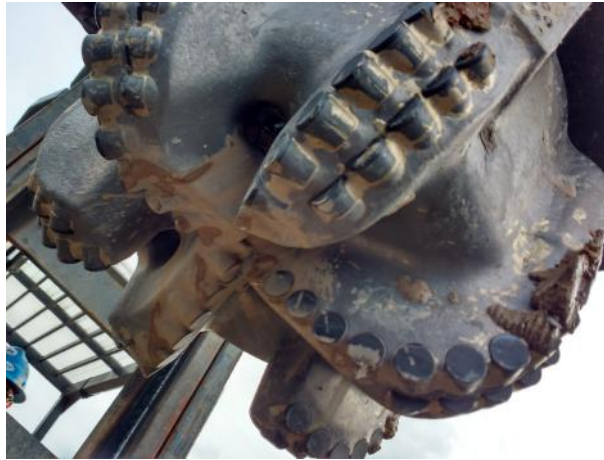
Figure 3.5: 12.25 fixed cutter bit with polycrystalline diamond compact (PDC) cutters that was used in the field tests performed with the 9.5in vibration-assisted tool at Genesis Test and Training Facility.
