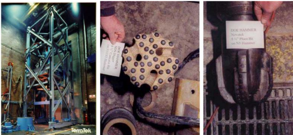
Figure 1.9: Terratek test facility where the tests with the SDS Digger Hammer were performed and two of the bits used in these tests. [4].
