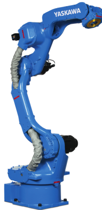
Figure 1.5: Example of serial type robotic manipulator chosen to be used in the in situ hard coating processes by the EMMA team. . [4]
