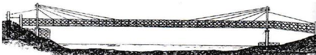
Figure I. 2: First proven constructed cables-stayed bridge: Kings Meadow Bridge, 1817 (STEPHENSON, 1821 apud SVENSSON, 2012).
