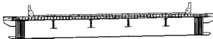
Figure I. 8: Composite steel-concrete cross-section: two main plate girders (BATTISTA, 2013).
