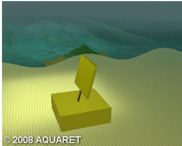
Figura 3-3 – Oscillating wave surge converter (EMEC, [s.d.]
