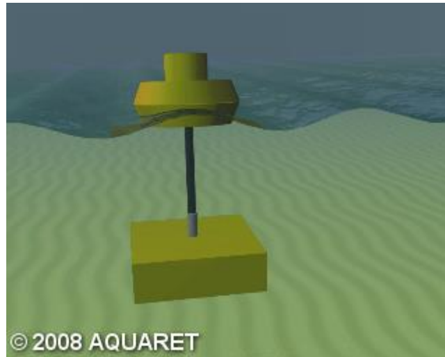
Figura 3-5 – Point absorber (EMEC, [s.d.]
