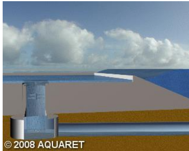
Figura 3-4 – Overtopping device (EMEC, [s.d.])
