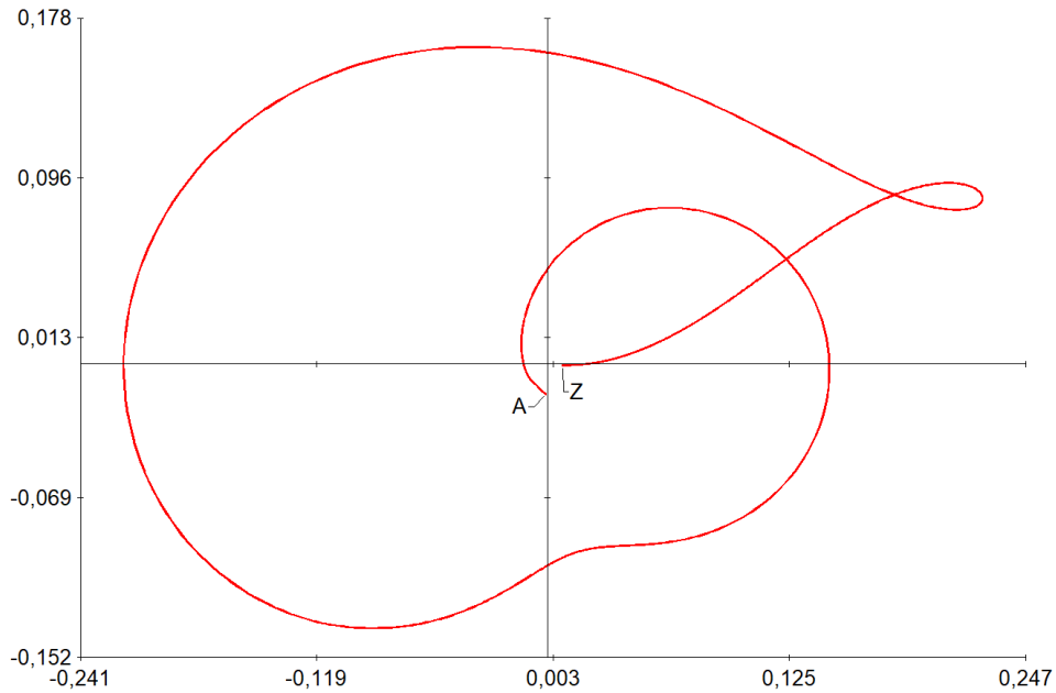
Figure 4.6: Uncompensated Nyquist Diagram for The Second PSS Design.
