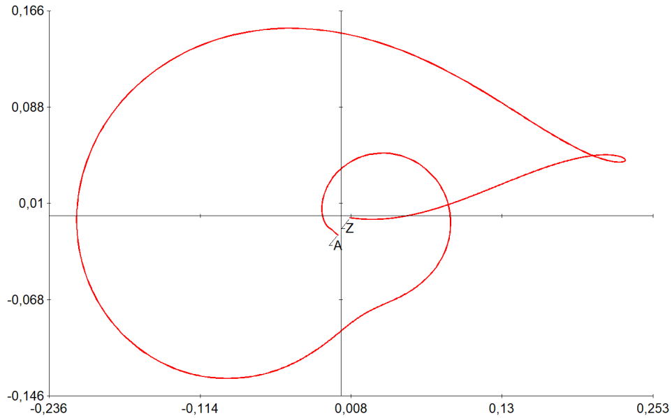
Figure 4.14: Uncompensated Nyquist Diagram for The Second PSS Design.
