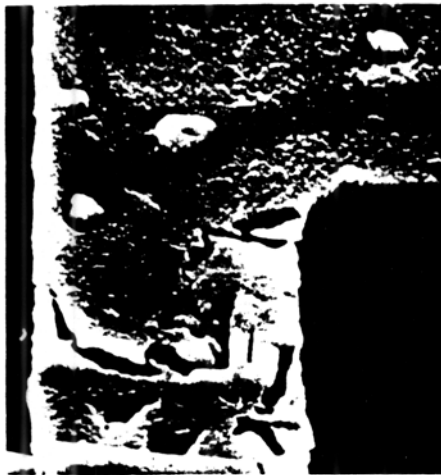
Fig. 1. 1 mil wide Al stripe I/C conductor which has failed due to electromigration.
