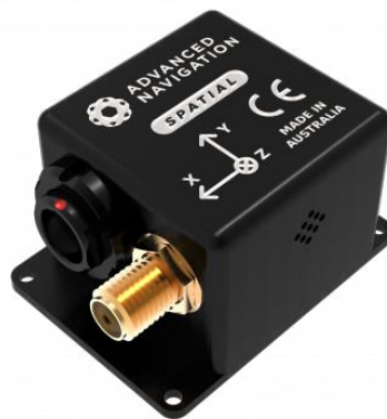
Figura 3.2: IMU Advanced Navigation Spatial .
