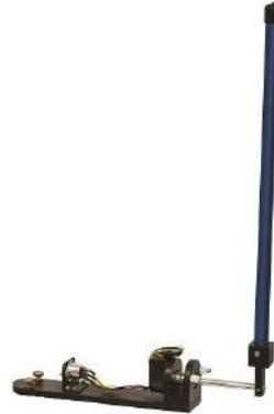
Figura 5.8: Rotary Inverted Pendulum Module.
