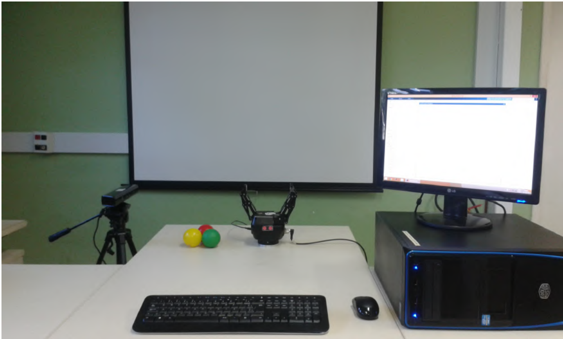
Figure 4.2: Experimental setup for visual servoing experiments.
