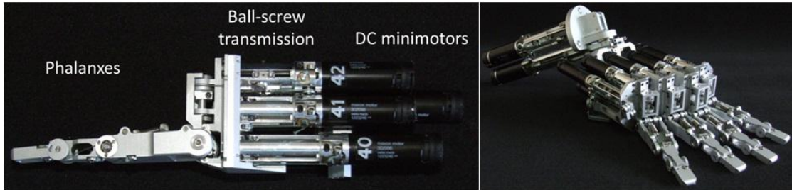
Figure 2.6: On the left: prototype of the 3-axes unit. On the right: assembly of the fingers, all fingers actuators being integrated in the palm.
